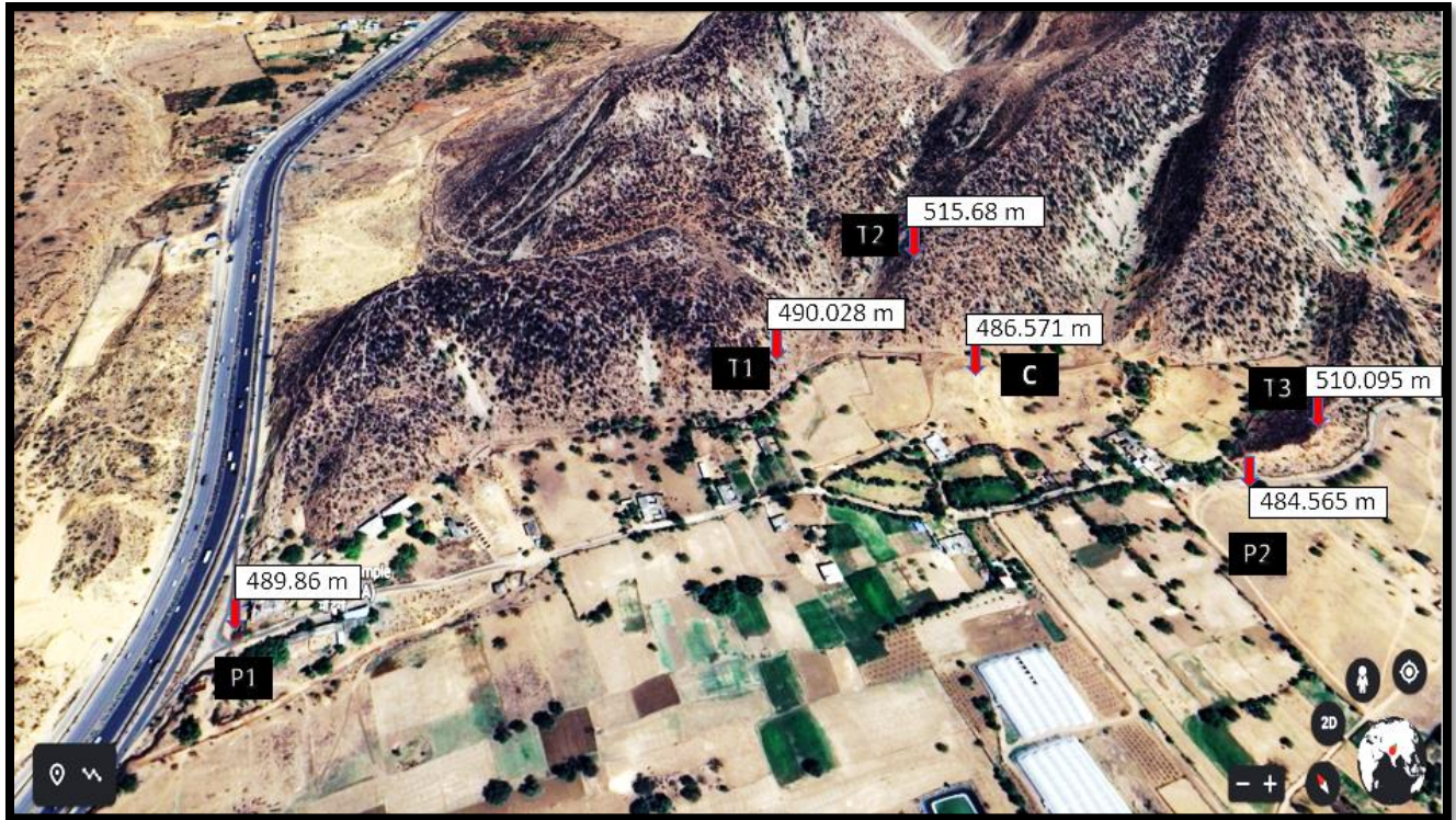
Satellite Map of Survey Camp Site with the RL of different Stations
